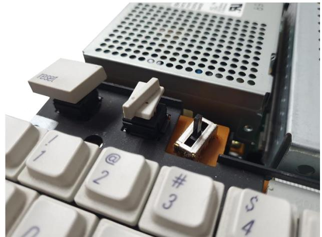
7. Flip the keyboard up and unplug it from the motherboard by pulling the connector up and out of the box header. Set the keyboard aside (you may want to take the opportunity to give the keyboard a good clean):
