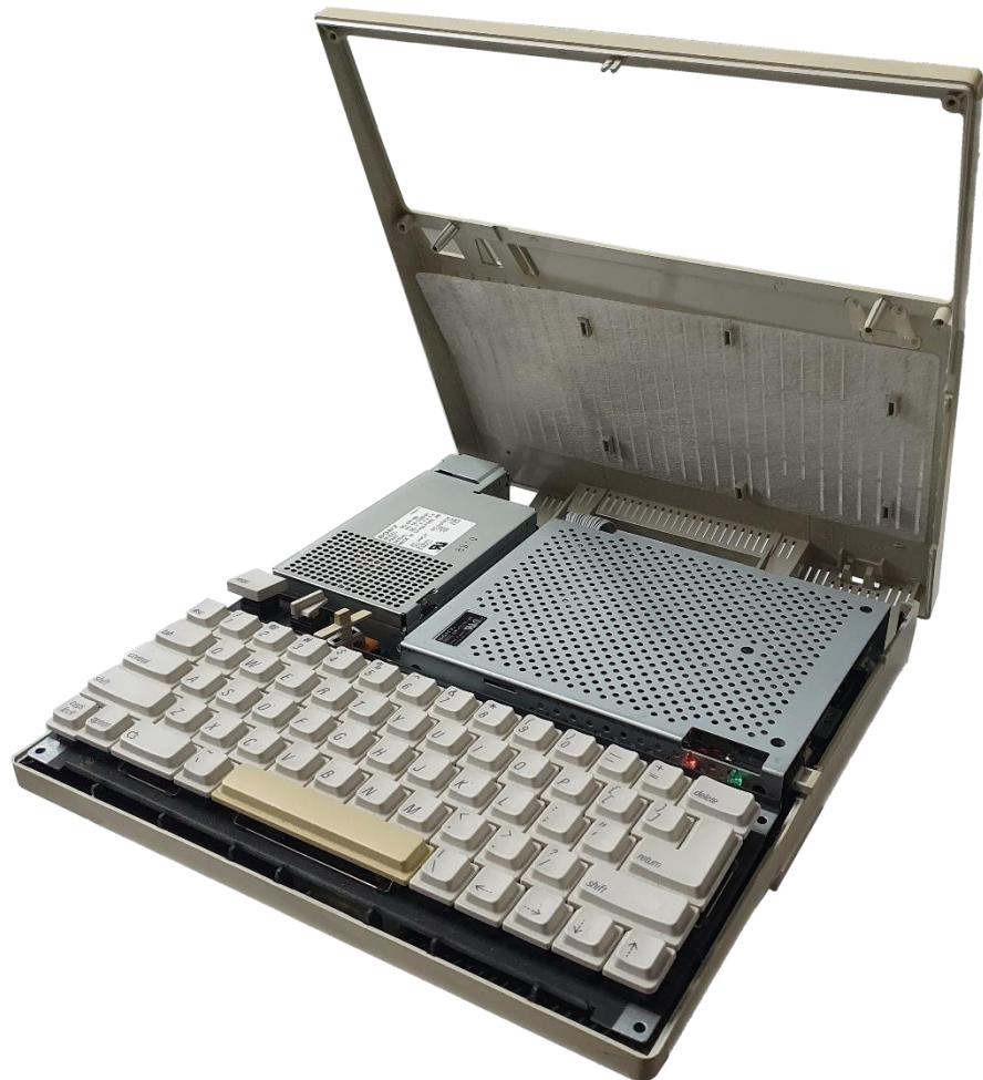
6. So as it does not fall off and become lost, it may be worth removing the volume slider cap from the slider shaft before removing the keyboard:
