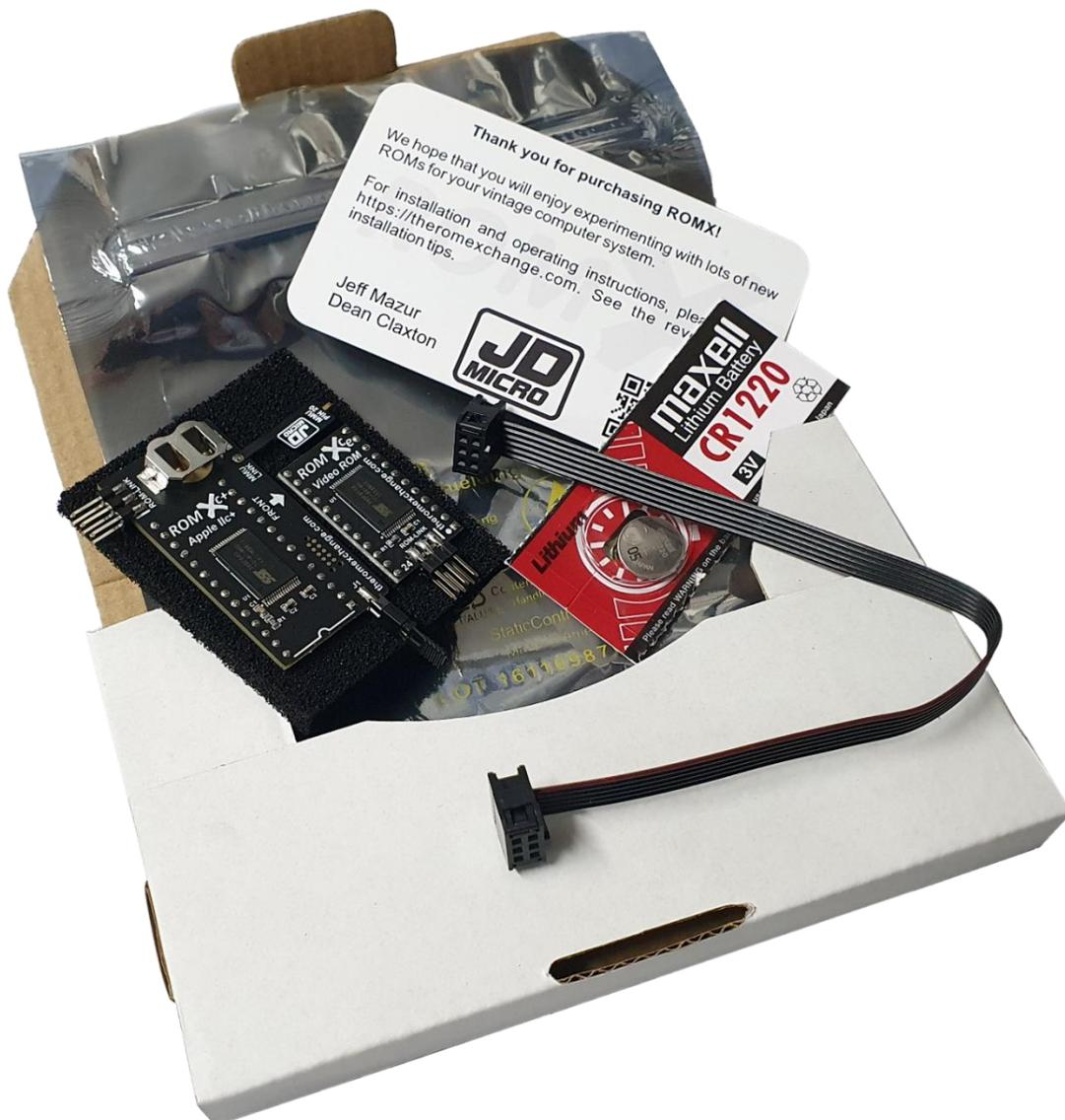
Before removing your ROMX modules from the ESD compliant packaging, please study the ESD Prevention section of this installation guide.
