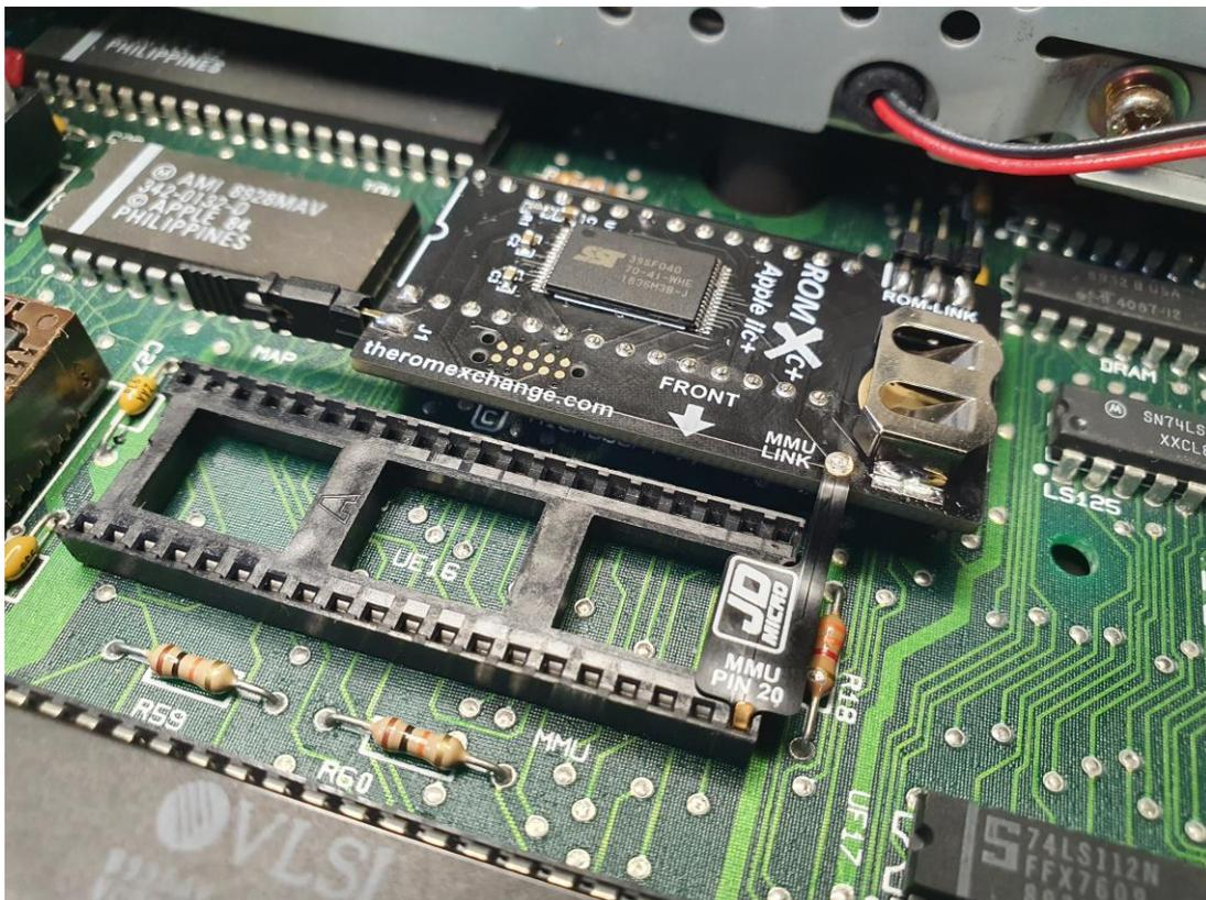
13. Reinstall the MMU over the top of the MMU-Link flex cable, ensuring that the MMU is fully seated :
