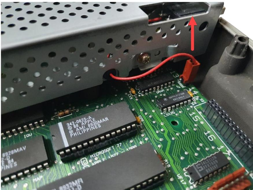
10. Lift the disk drive out vertically and place it aside.
