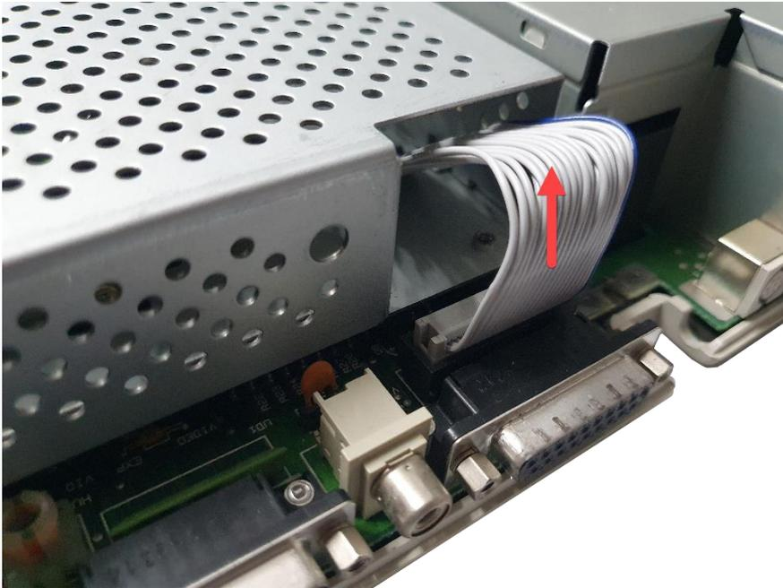
9. Unplug the disk drive eject switch cable by pulling the connector up from the header :
