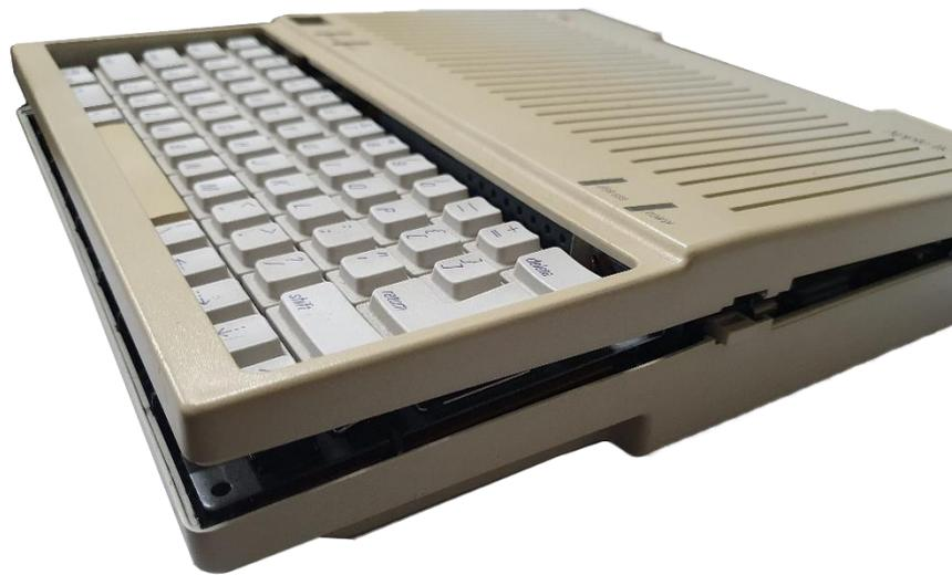
5. Once released the upper shell can be slid back and lifted away, giving us full access to the internals. Take care as you work the top shell away from the lower shell:
